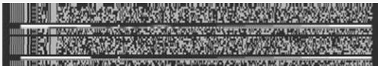
Figure 32-5. The vertical blanking interval of NBC Europe.
