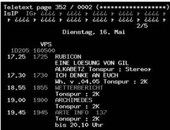
Figure 32-6. Text hidden in the vertical blanking interval
